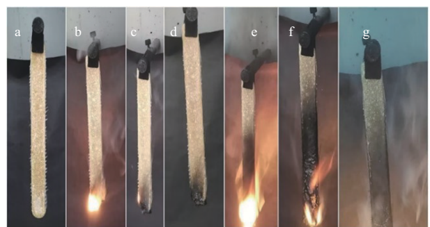
(a) Primary ignition 0 s; (b) Primary ignition 10 s; (c) After primary ignition 5 s; (d) After primary ignition 8 s; (e) Secondary ignition 10 s;
