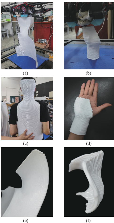
背部支具: a—打印过程; c—穿戴测试; e—支具细节
