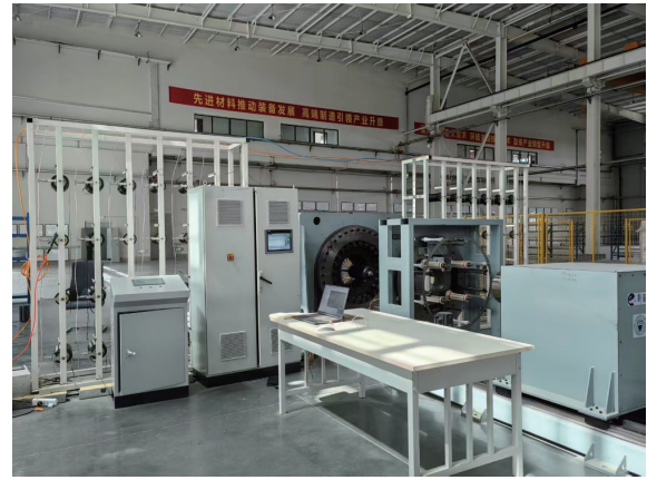
(a) Multi-filament carbon fiber winding equipment diagram
