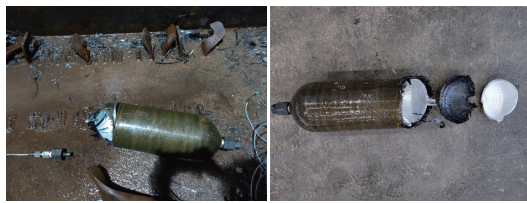
(a) SFW hydrogen storage cylinder (b) MFW hydrogen storage cylinder
