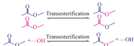
(d) Mechanism of transesterification reaction during hot pressing process
