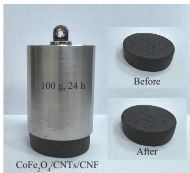
(c) Aerogel before and after carrying 100 g weight for 24 h
